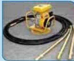
Concrete vibrator (gasoline)
